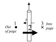
Front view, again. On the left side of the wire (point 1) the mag field, B, is out of the page (imagine a pin pushed "through" the page). On right of wire (point 3), B is into page. In front of the wire (point 2) *B* is to the right, etc.
