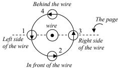
Here is the same wire viewed from above. The dot in the wire means the current is toward you. Notice B is counterclockwise (CCW) around the wire. Also, the dashed line represents "the page" for the next diagram (at the right), which is a 2D drawing on this piece of paper.
