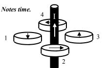
In the lab we saw compasses prove that current in a wire creates a circular magnetic field (B). In this case the current is up (notice the "I" on the wire). Put your right thumb up and your fingers curl in the direction of the compasses.
