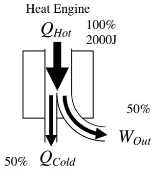
Notice that the  $Q_H$  arrow is equal to the  $Q_C$  and  $W$  arrows. So  $Q_H$  is the whole and the others are the parts.  $W$  is the useful work done by the engine.  $Q_C$  is the heat that is not used, so is “wasted” and is the inefficiency of the engine. This engine is 50% efficient.
