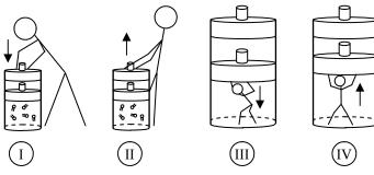
In the first two diagrams, Slim Jim is pushing or pulling on the piston from the outside. In the second two diagrams, we imagine Slim Jim is the gas inside the cylinder, also known as the system. The arrows show the direction the piston moves. Remember: when a gas is compressed it's molecules speed up due to the collision with the piston, raising its temperature and internal energy.
