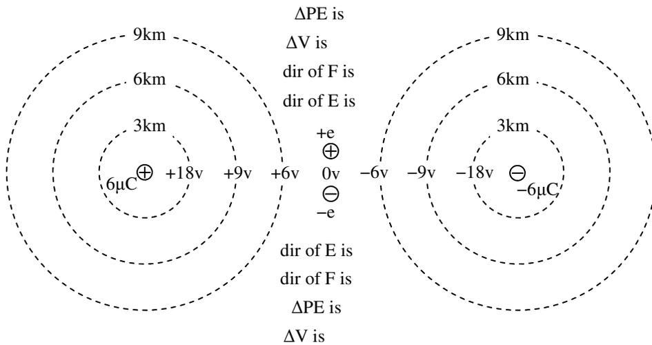
I have now put all of the potentials (voltages) on the diagram for you, to simplify the following discussion. Notice that I have placed a +e and a -e at the 0V point. The +e stands for a positive elemental charge: a proton. The -e stands for a negative elemental charge: an electron.
