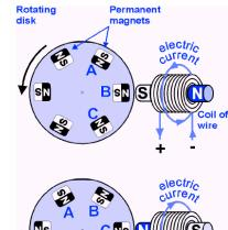
Motor or Generator? Depends on if electricity is going in or out.
