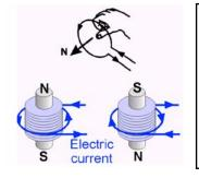
**Right-hand rule:** To find the north pole of an electromagnet, simply wrap your right hand fingers in the direction of the electric current (from + to -). Your thumb will point in the direction of the electromagnet's north pole.
