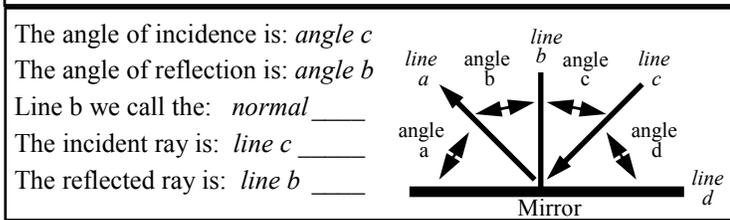
If the angle of incidence is 50°, what is the angle of reflection?
